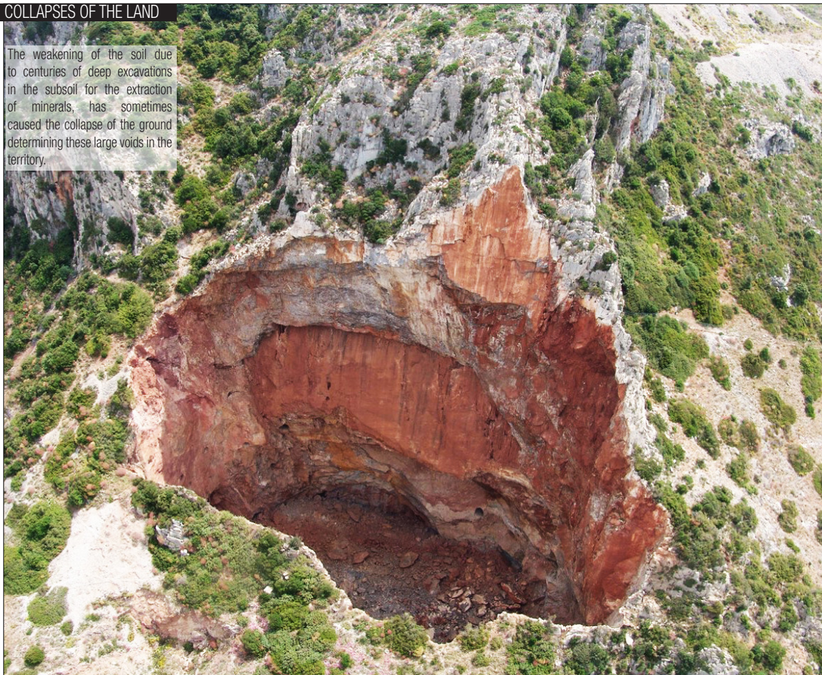
Collapse occurred at the mine of Masua due to the weakening of the soil because of mining activity
